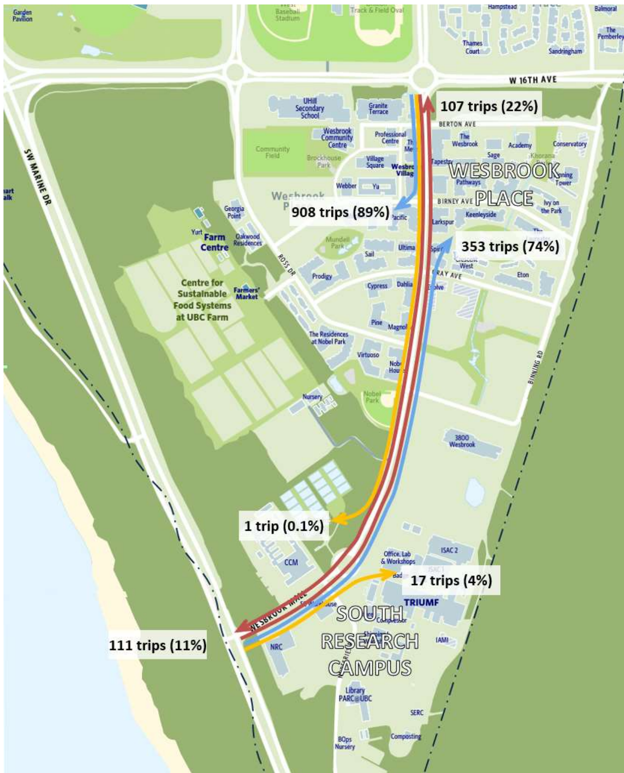
Figure 4.3: Travel Patterns on Wesbrook Mall between 16 th Avenue and SW Marine Drive
